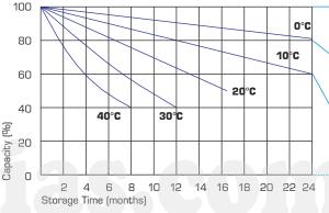
Supplementary charge required (Carry out supplementary charge before use if 100% capacity is requires)
