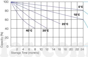
Supplementary charge required (Carry out supplementary charge before use if 100% capacity is requires)
