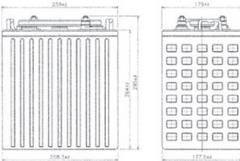
6V 260 Ah at 20 houres discharge 3 ca. 33.0kg +/- 3% 6.50 - 6.70V Discharge: Charge: Storage:  $0^{\circ}C - 50^{\circ}C$ - 20°C – 60°C - 20°C – 60°C 20°C ± 5°C Valve Regulated Lead Acid (VRLA) batteries can be stored for more than 3 months at 20°C. Please charge batteries before using. Dual Fit
